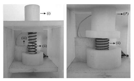
Figure 4. Spring Button's interior side view on Panel E and interior side view with the cylinder pressed down on Panel F. (i) cylinder; (i\*) cylinder pressed down; (ii) steel spring; (iii) microswitch.
