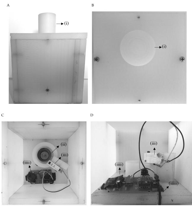
Figure 2. Spring Button interior top view on the Panel C and interior side view on the Panel D. (ii) steel spring (the spring is removable); (iii) microswitch; (iiii) mouse's circuit board; (iiiii) USB cable.
